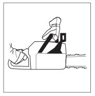
6 The way the chain brake is triggered, either manually or automatically, depends on the force of the kickback and the position of the chain saw in relation to the object that the kickback zone of the bar strikes.
